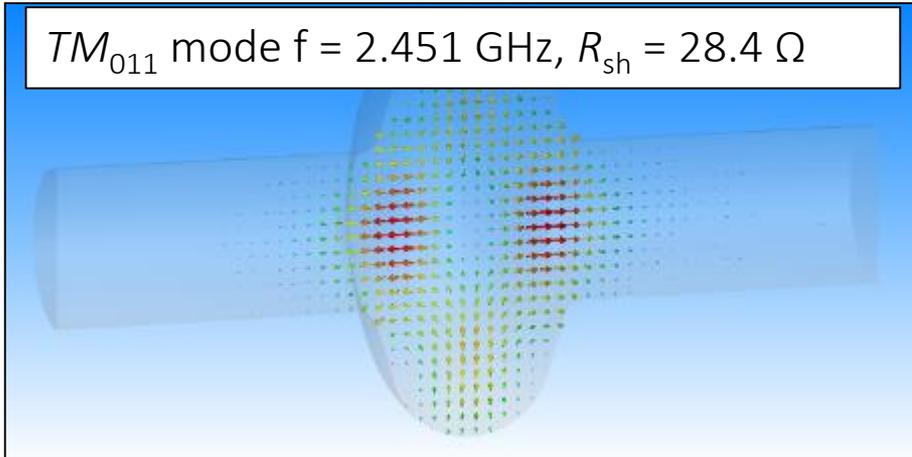
$$f_{c, TM01} = \frac{c}{2\pi} \cdot \frac{x_{mn}}{R} = 2.94 \text{ GHz} > f_{TM011}$$
