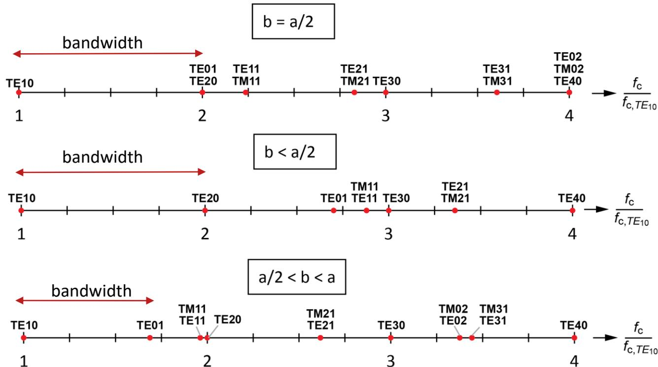
Cutoff frequencies in a rectangular waveguide for the first  $TE$  and  $TM$  modes (normalized to first  $TE_{10}$  cutoff frequency) depending on the ratio of the waveguide height to the waveguide width  $b$ . Mode degeneracies may occur.
