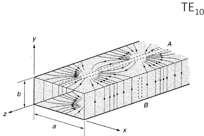
Surface current distribution for the  $TE_{10}$  mode at a fixed time. The mode moves in  $z$  direction.
