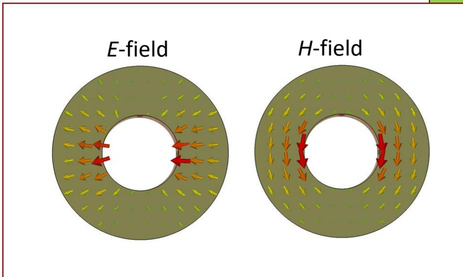
cutoff wavelength below which *TE*<sub>11</sub> mode can propagate
