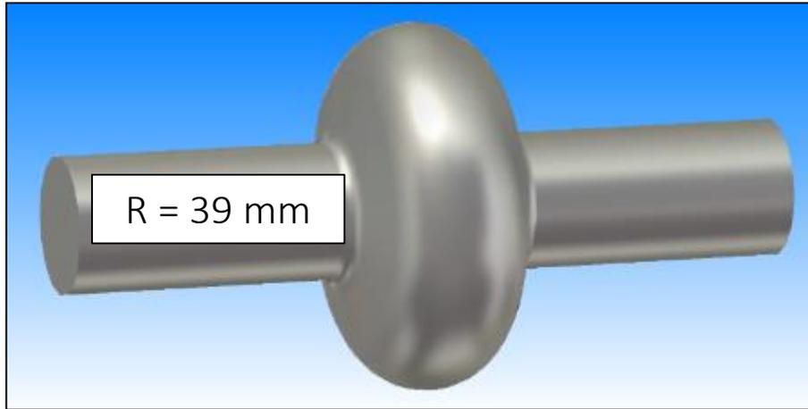
$TM_{010}$  mode  $f = 1.302 \text{ GHz}$ ,  $R_{sh} = 105.6 \Omega$
