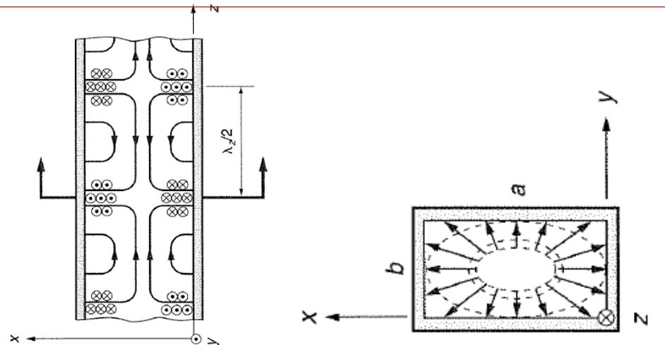
E-field (solid) lines and H-field (dashed) lines at a fixed time.
