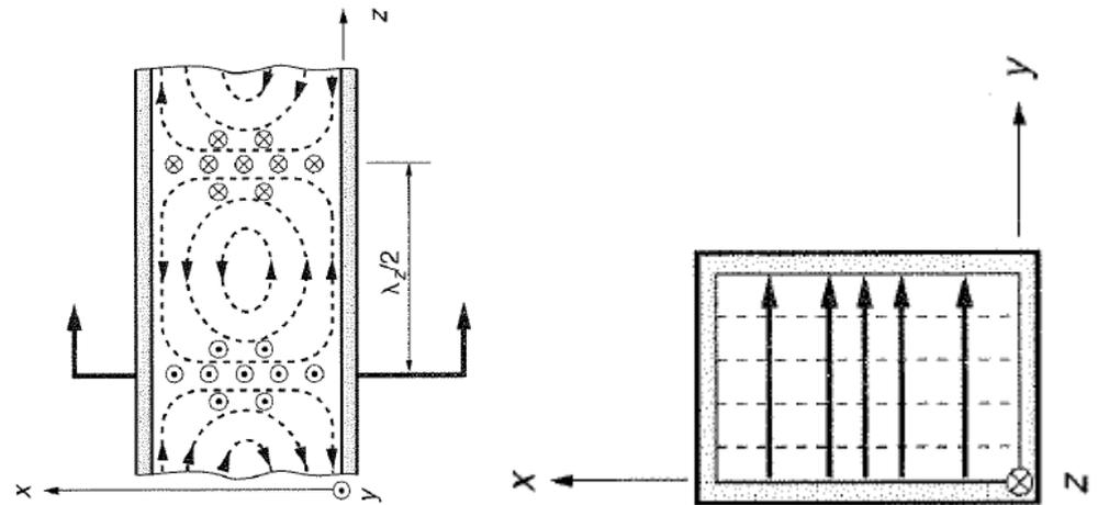
E-field (solid) lines and H-field (dashed) lines at a fixed time.
